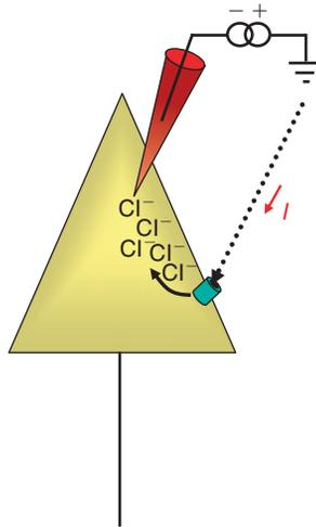
f0060 **FIGURE 3.11**  $V_m$  is hyperpolarized by applying a negative current via an intracellular electrode.
