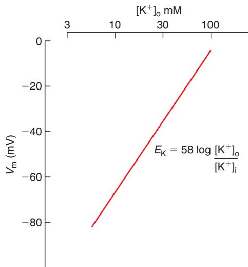
f0045 **FIGURE 3.8** Theoretical diagram of  $E_K$  versus the external concentration of  $K^+$  ions ( $[K^+]_o$ ).  $E_K = (RT/zF) 2.3 \times \log([K^+]_o/[K^+]_i)$ .
