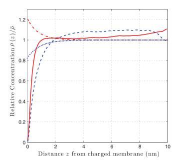
FIG. 3. (Color online) Monte Carlo predictions for the relative concentrations of potassium  $\rho_{\rm K}(z)/\bar{\rho}_{\rm K}$  (solid, red) and chloride  $\rho_{\rm Cl}(z)/\bar{\rho}_{\rm Cl}$  (dashed, blue) ions at a distance *z* (nm) from the charged cytosolic leaflet of a lipid bilayer are plotted along with the Gouy-Chapman predictions (40) for the normalized potassium  $K_{\rm GC}(z)$  (dot-dash, red) and chloride  ${\rm Cl}_{\rm GC}(z)$  (dots, blue) concentrations.
