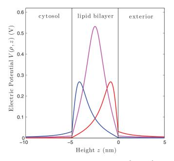
FIG. 2. (Color online) The electric potentials  $V_w^{\ell}(\rho, z)$ ,  $V_\ell^{\ell}(\rho, z)$ , and  $V_c^{\ell}(\rho, z)$  [(15), (16), and (17)] (V) for  $\rho = 1$  as a function of the height *z* above the phospholipid bilayer for a unit charge q = |e|in the phospholipid bilayer at  $(\rho, z) = (0, -4.5)$  (left curve, blue), (0, -2.5) (middle curve, magenta), and (0, -0.5) (right curve, red). Distances and permittivities are as in Fig. 1.
