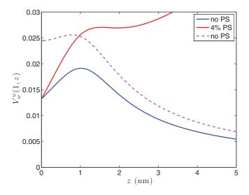
FIG. 7. (Color online) The potential  $V_w^w(\rho, z)$  [V, (59)] at the point  $(\rho, z)$  due to a charge q = |e| on the z axis at (0, h) above a three-slab phospholipid bilayer that is neutral (lowest, solid, blue) or has a 4 mol % layer of PS on its cytosolic leaflet (upper, solid, red). Both  $\rho$  and h are 1 nm. The potential (9) of a charge above a single neutral lipid slab without head groups is plotted as a dashed magenta curve to illustrate the effect of the layers of head groups.
