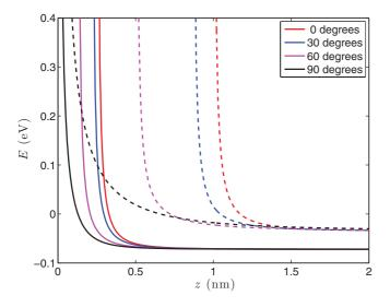
FIG. 6. (Color online) The energy (44) of a zwitterion in salty water a distance z from a lipid slab. The four lower, solid curves are for a molecule consisting of a point charge q' = |e| separated by 0.5 nm from a charge q'' = -|e|; the four upper, dashed curves are for a molecule consisting of a point charge q' = 2|e| separated by 2 nm from a charge q'' = -|e|. Within each quartet the molecules from right to left make angles of 0°, 30°, 60°, and 90° with the vertical.
