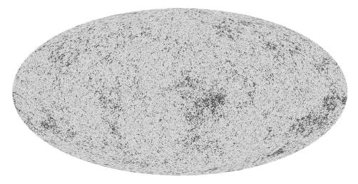
Figure 8.2 CMB temperature fluctuations over the celestial sphere as measured by the Planck satellite. The average temperature is 2.7255 K. White regions are warmer and black ones colder by about 0.0005 degrees. © ESA and the Planck Collaboration.
