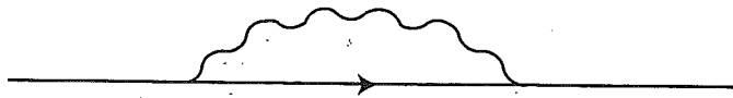
Figure 11.6. The one-loop diagram for the electron self-energy function. As usual, the straight line represents an electron; the wavy line is a photon.
