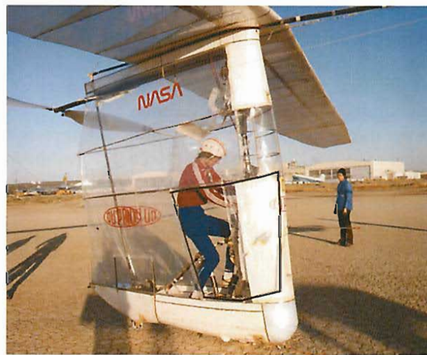
Figure 1.5 Bryan Allen, about to pedal the Gossamer Albatross , with its 96-foot wingspan. It weighed only 66 pounds. Allen was both the pilot and the engine. (Photo courtesy of NASA.)
